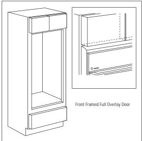
Monogram ovens are installed directly into a wall or wall oven cabinetry, 30" minimum width. The front surface of the ovens will be nearly flush with surrounding cabinetry. To obtain optimal appearance, cabinet cutouts must be exact. The examples shown here illustrate typical styles of 30" cabinets and oven fit. Installation instructions for each of these basic cabinetry styles are provided in this section.
